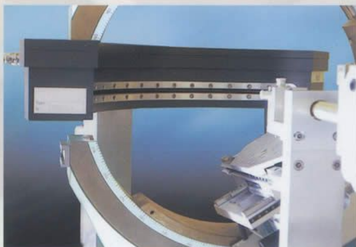
Curved Positions Sensitive 120° detector
