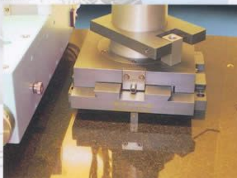
X-Y and rotatable stage for tube shield
