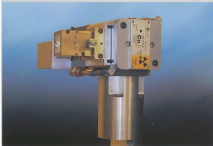
Parallel-beam monochromator using a Göbel mirror
