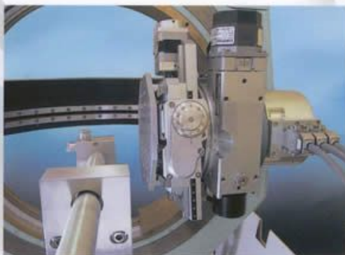
Motorised sample holder X-Y-Z translation
