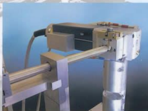
X-ray tube rotatable between line and point focus
